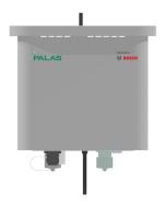
The ECoB (Environmental Connected Box) was developed to better understand the relationships between emission sources and the environment. By continuously transmitting locally-sourced environmental parameters to a cloud platform, the ECoB facilitates real-time analyses and applications. The Bosch Cloud Services allow for the retrieval of the datasets at one's convenience, facilitating advanced simulations.
